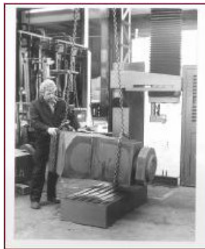
▲ Swing radial arm out of the way to lower heavy workpiece by crane
